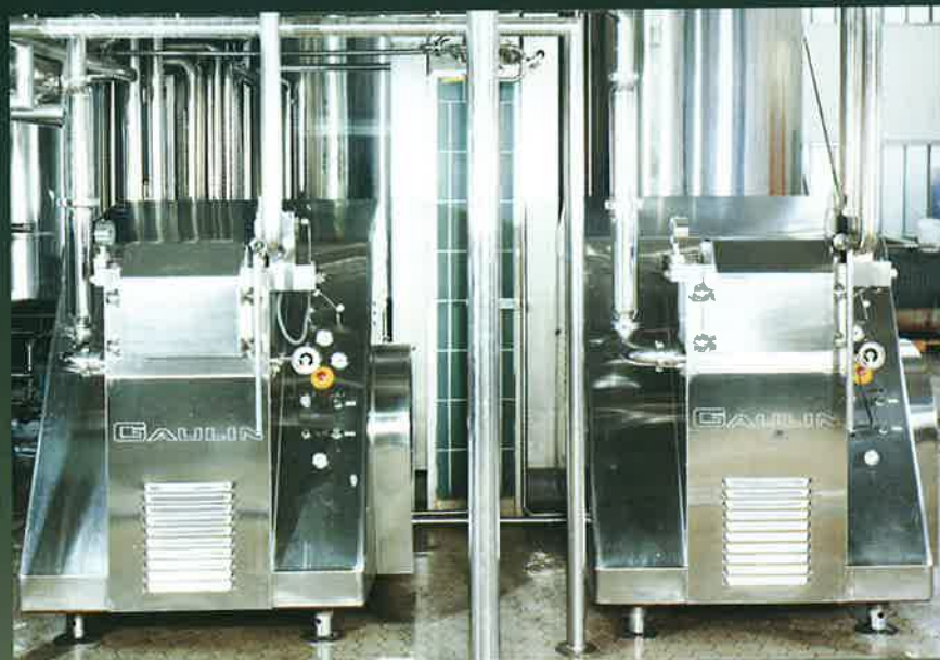
△ Model MC 45-5TBS High-pressure homogenizer for the production of fruit nectars in a 15000 l/h installations
