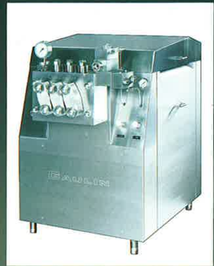
△ Model MC7 high-pressure homogenizer for small and medium production capacities in the fruit and vegetable industry.
