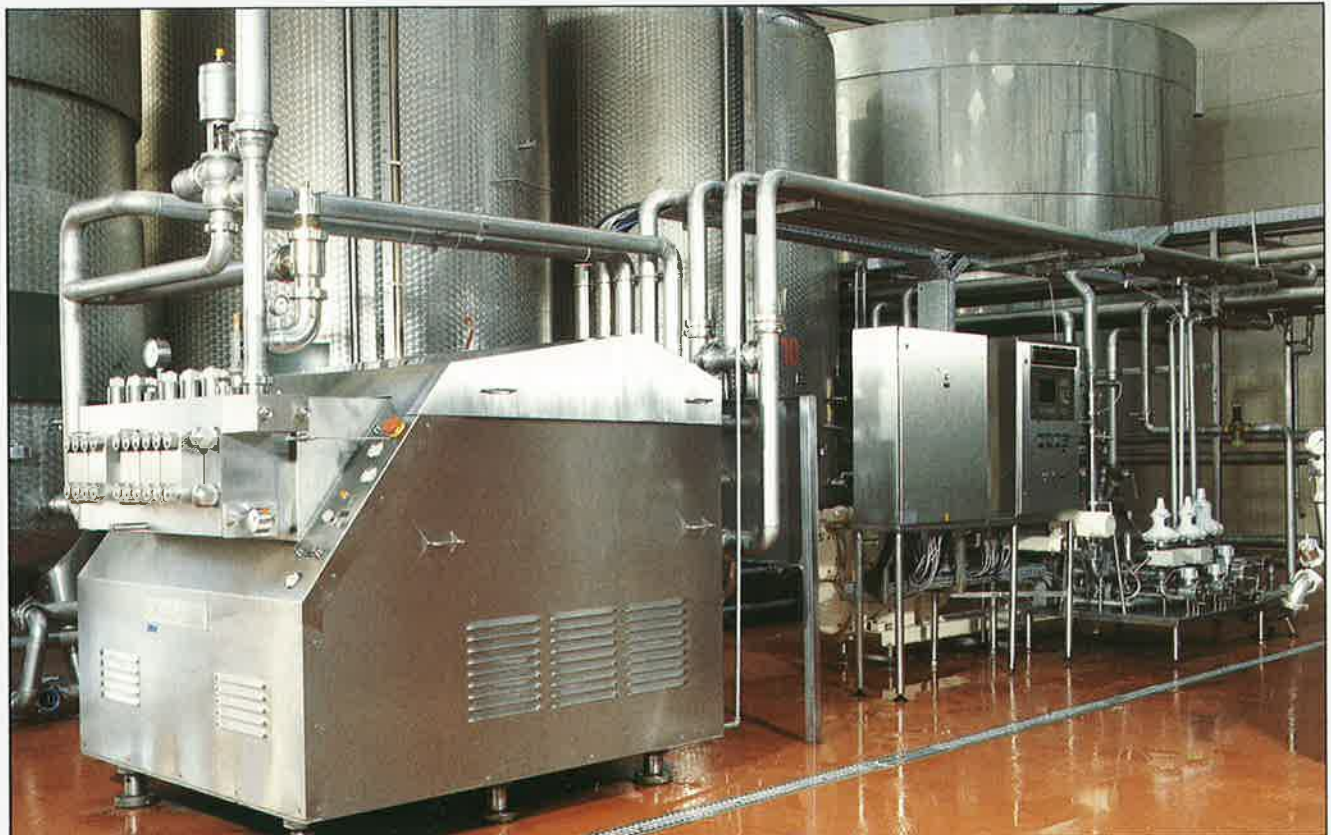
▽ High-Pressure Homogenizer MC 120-5TBS a 5-plunger machine for capacities of up to 40.000 l/h.
