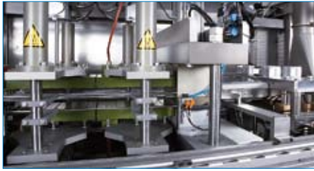
Pre-heating and forming station
